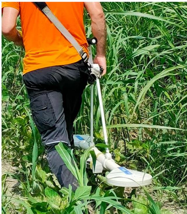
Figura 2 - Elettromagnetometro Profiler EMP-400 (GSSI, USA)
